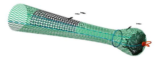
Figure 6 Square mesh panel inserted in a diamond mesh codend (Copyright 2004 reproduced with permission of FRS, Aberdeen).
