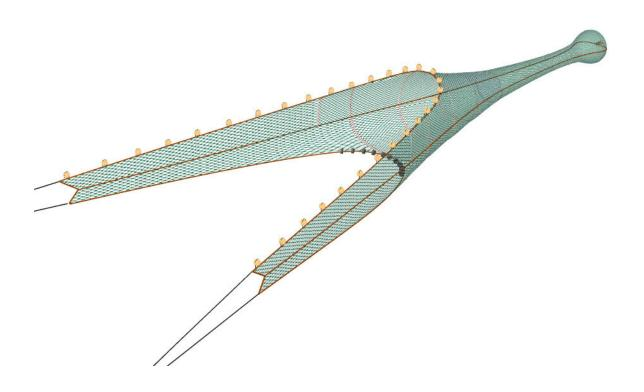
Figure 7. Cutaway trawl with set back headline (Copyright 2004 reproduced with permission of FRS, Aberdeen).
