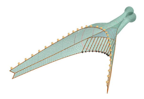
Figure 4 Horizontal separator trawl fitted with guiding ropes to encourage separation of cod from Nephrops (Copyright 2004 reproduced with permission of FRS, Aberdeen).
