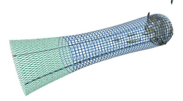
*Figure 8. Full square mesh codend (Copyright 2004 reproduced with permission of FRS, Aberdeen).*
